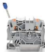
Push-in termination of solid and ferruled conductors
